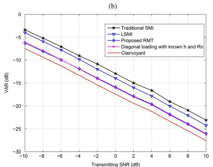
Fig. 5. SNR, MSE and VAR in the beamforming problem of wireless communications: transmitting SNR varies from -10 to 10 dB,  $M = 20$ ,  $N = 30$ .
