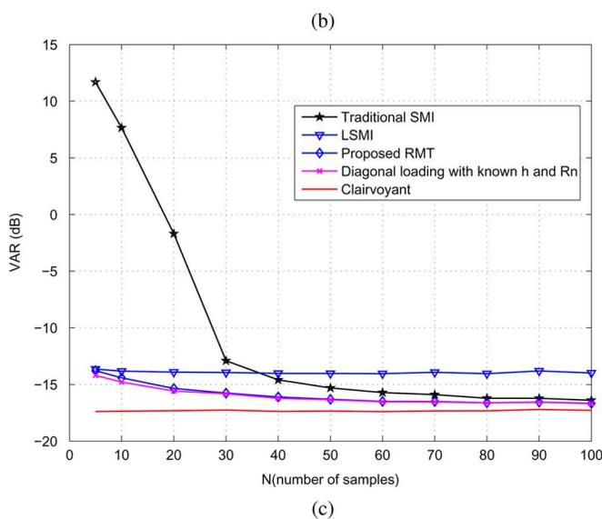
Fig. 4. SNR, MSE and VAR in the beamforming problem of wireless communications: transmitting SNR is 0 dB,  $M = 20$ ,  $N$  varies from 5 to 100.
