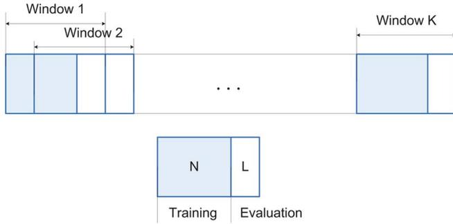
Fig. 2. The rolling-window procedure: In the  $k$ th window, the first  $N$  observations are used as the training samples and the following  $L$  observations are used for evaluation. The window shifts until the end of the data set.
