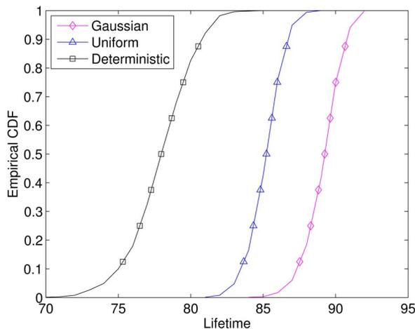
Fig. 9. Empirical CDF of the network's lifetime using the stochastic random model where there is an extra random energy consumption over time.
