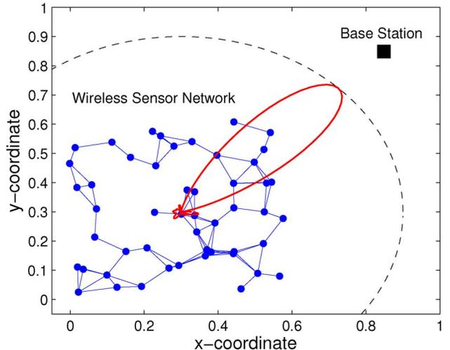
Fig. 1. Beamforming scenario between the nodes and the far-away base station.
