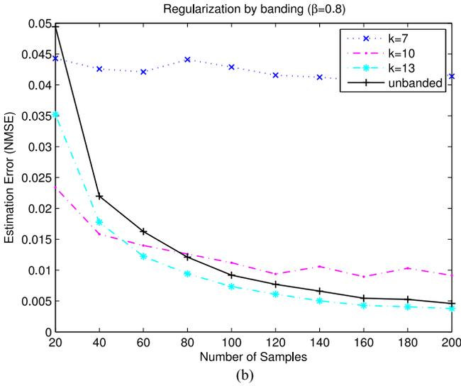
Fig. 5. NMSE of the Tyler's estimator versus the number of samples  $N$  under a banded Toeplitz structure of bandwidth  $k$ : (a) population parameter  $\mathbf{R}_0 = \mathbf{R}(0.4)$  (fast decay), (b) population parameter  $\mathbf{R}_0 = \mathbf{R}(0.8)$  (slow decay).
