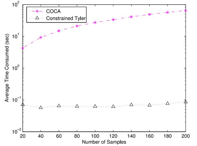
Fig. 8. Average time (in seconds) consumed by COCA and constrained Tyler's estimator as the number of samples  $N$  varies from 20 to 200.
