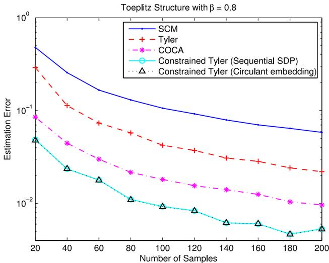
Fig. 1. Estimation error (NMSE) versus the number of samples  $N$  of different estimators under the Toeplitz structure of the form (71).
