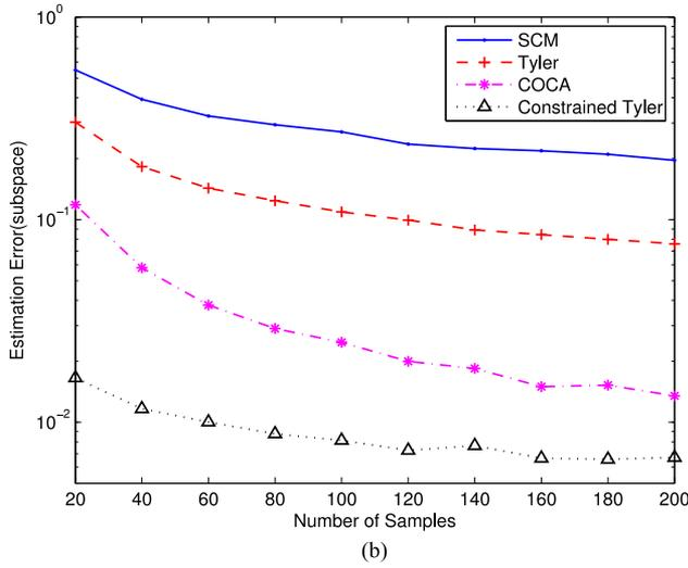
Fig. 7. The estimation error of different estimators versus the number of samples  $N$  under the DOA structure: (a) NMSE, (b) estimation error of the noise subspace given by different estimators evaluated by (75).
