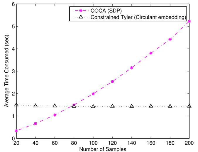
Fig. 4. Average time (in seconds) consumed by COCA and constrained Tyler's estimator as the number of samples  $N$  varies from 20 to 200.
