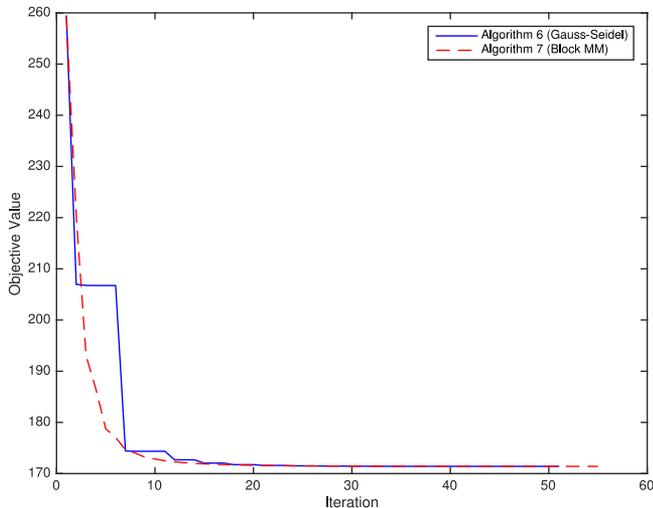
Fig. 10. Convergence comparison of Algorithm 6 and 7 under the Kronecker structure ( $N = 4$ ,  $\mathbf{A}_0 = \mathbf{I}$ ,  $p = 10$ ,  $\mathbf{B}_0 = \mathbf{R}(0.8)$ ,  $q = 8$ ).
