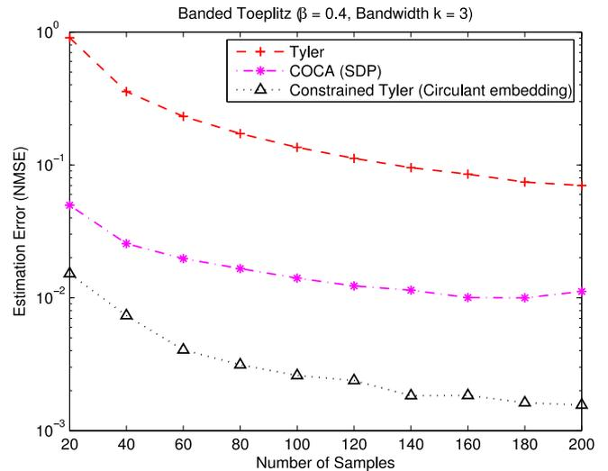
Fig. 3. Estimation error (NMSE) versus the number of samples  $N$  of different estimators under the banded Toeplitz structure.
