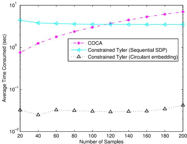
Fig. 2. Average time (in seconds) consumed by COCA and the constrained Tyler's estimator via sequential SDP (Algorithm 1) and circulant embedding (Algorithm 2) as the number of samples  $N$  varies from 20 to 200.
