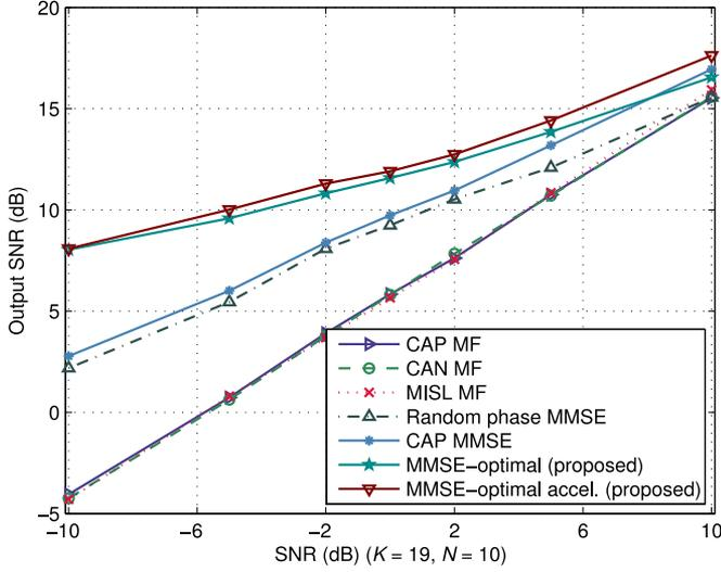
Fig. 2. Output SNR of SISO channel estimates with different unimodular training sequences. The results are averaged over 200 Monte Carlo simulations.
