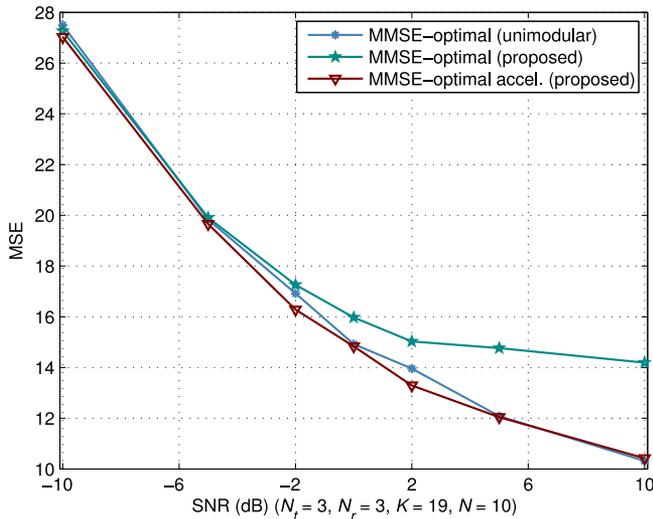
Fig. 6. MSE with different low PAR training sequences for MIMO channels.  $\text{PAR} = \{5, 5, 5\}$  with equal power for three antennas. The results are averaged over 100 Monte Carlo simulations.
