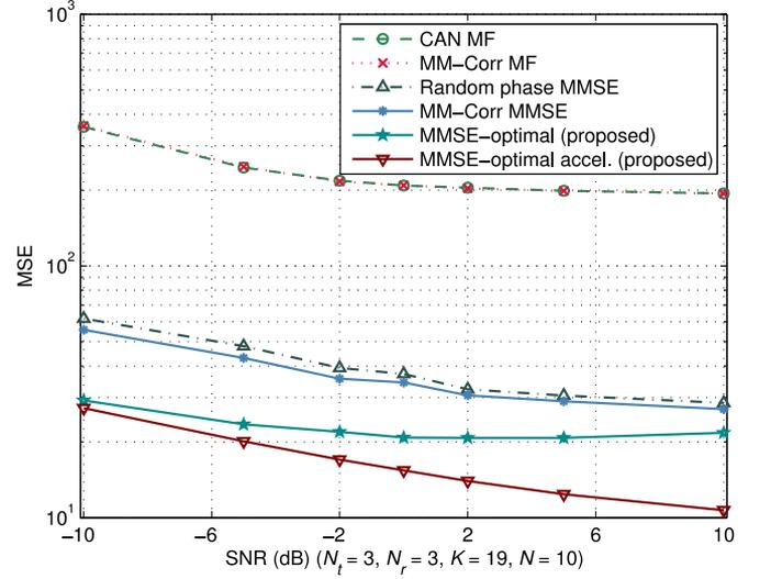
Fig. 4. MSE of MIMO channel estimates with different unimodular training sequences. The results are averaged over 100 Monte Carlo simulations.
