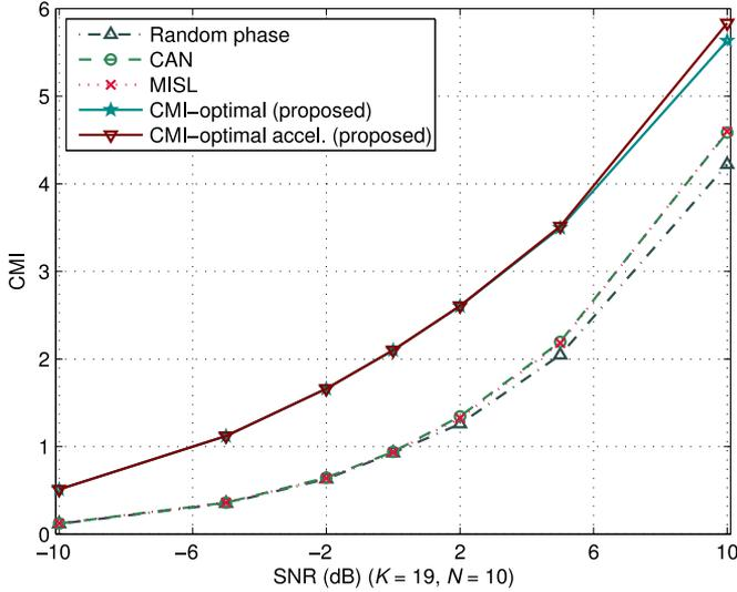
Fig. 3. The CMI with different unimodular training sequences for SISO channels. The results are averaged over 200 Monte Carlo simulations.
