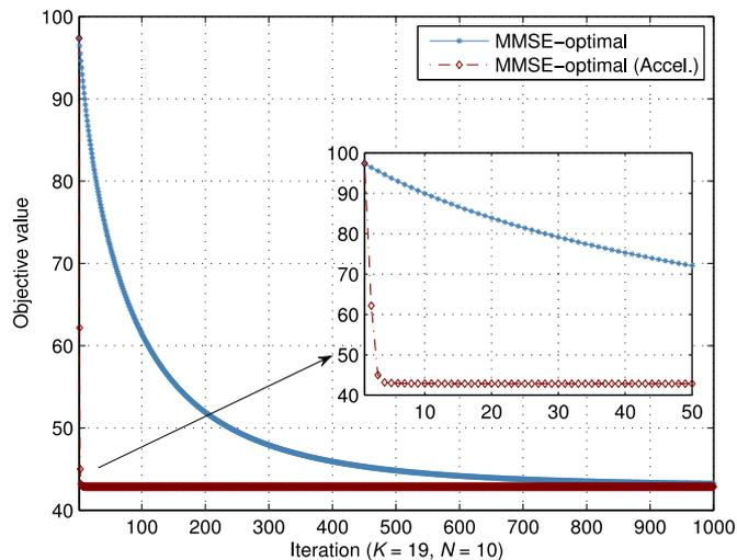
Fig. 10. Convergence of algorithms for optimal low PAR sequence design for MIMO channel estimation,  $N_t = 3$ ,  $N_r = 3$ , and SNR = -5 dB.
