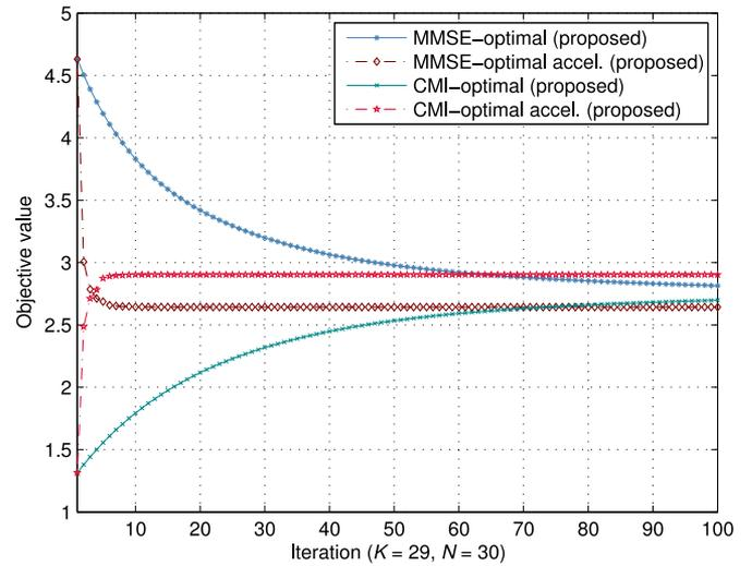
Fig. 8. Convergence of algorithms for optimal unimodular sequence design for SISO channel estimation,  $\text{SNR} = -5$  dB.
