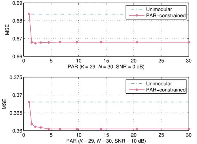
Fig. 7. MSE for SISO channel estimation with PAR-constrained sequences or unimodular sequences. The results are averaged over 100 Monte Carlo simulations.
