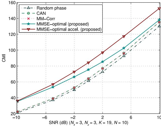
Fig. 5. The CMI with different unimodular training sequences for MIMO channels. The results are averaged over 100 Monte Carlo simulations.
