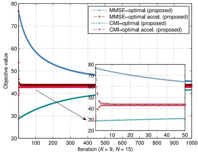
Fig. 9. Convergence of algorithms for optimal unimodular sequence design for MIMO channel estimation,  $N_t = 3$ ,  $N_r = 3$ , and SNR = -5 dB.
